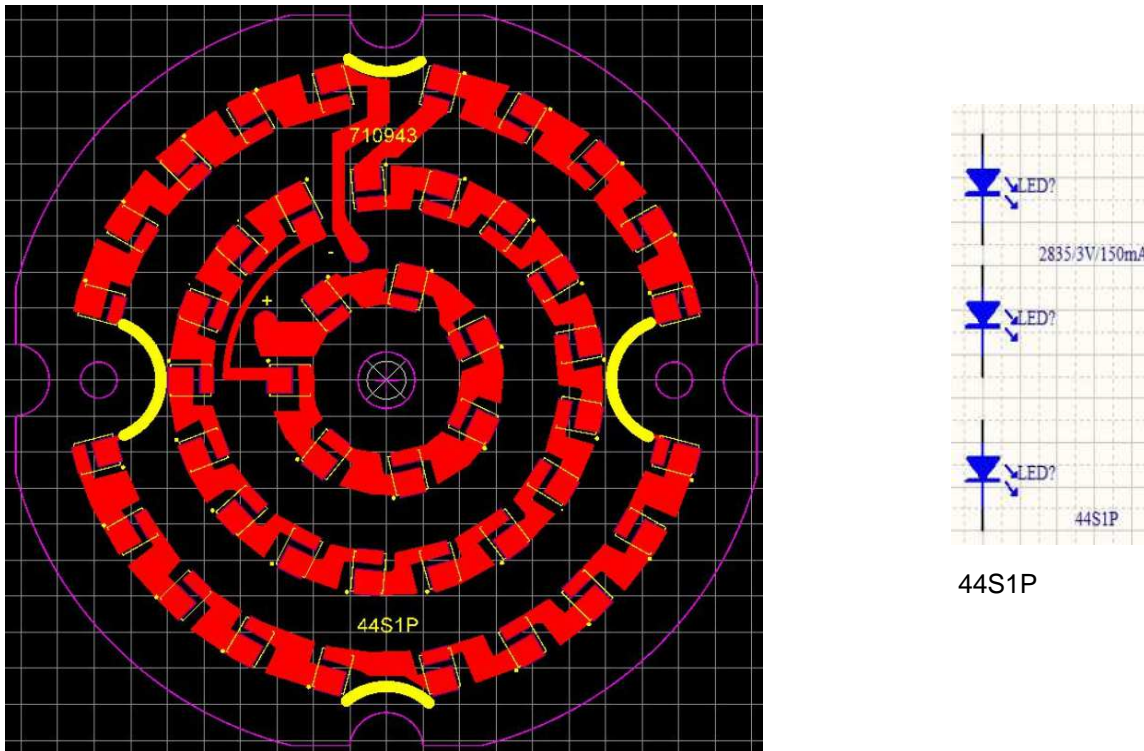
Illustration 3 - Schematic diagram and PCB layout of LED PCB of model Downlight 4"
