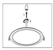
**Connect DC Power** Connect DC connector Turn connector cap 4.25" for A30114
