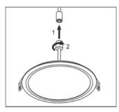
Connect DC Power Connect DC connector Turn connector cap
