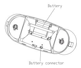
Unplug connector of battery Remove battery Plug new battery into battery connector Fix battery pack
